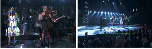
(a) Initialization (b) nearly lost target Figure 2: Fixed patch scale for a rapidly shrinking target( singer )
