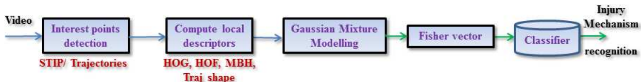
Figure 1. Overall Framework: Starting with an input video, first, interest points are generated and local descriptors computed. Codewords are obtained via GMM and Fisher vectors are generated from them to serve as feature vector. Finally, a SVM classifier is used to predict the action label.
