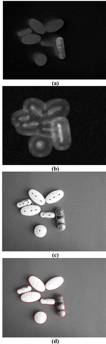
**Fig. 3.** Extraction of feature points and multi-location area descriptors for pill recognition: novelty map (a); multi-scale attention operator (b); feature point areas with pose descriptors (c); medication pills correctly recognized by the proposed algorithm (d).
