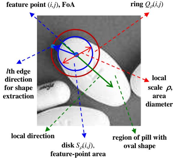
**Fig. 2.** Example of a feature-point area detected in an oval pill region.
