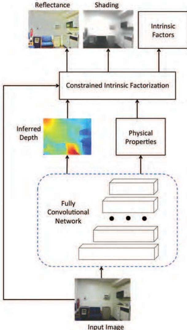
Figure 2. The full intrinsic pipeline. First, fully convolutional nets predict physical properties from the input image. The input image and FCN outputs are then fed into the constrained factorization stage. The decomposition is jointly optimized over reflectance, shading, and other intrinsic factors.
