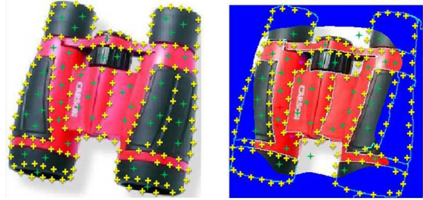
Figure 3. Left panel shows example of non-uniform spatial sampling. Right panel shows example of non-uniform spatial sampling + saliency detection. Sampling from the salient boundary are shown in yellow and sampling inside the region are in green.
