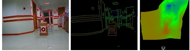
Figure 3. Edge reconstruction in a typical hallway with low amount of distinguishable features. From left to right: edge detection, edge depth and off-camera surface fitting.
