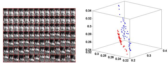
Figure 8. Effectiveness of discriminative low-rank learning. The positive (first fifty) and negative (the rest) samples are shown in the left. The reconstructed positive (red) and negative (blue) samples over the first three basis vectors are shown in the right.
