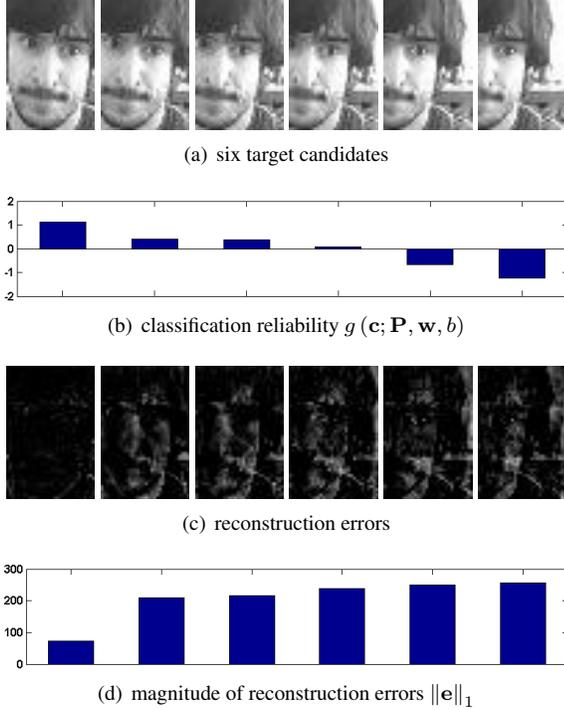
Figure 3. Six target candidates are shown in (a) and their classification reliability values are shown in (b). The reconstruction errors of the six target candidates are shown in (c), where the darker pixel indicates the smaller value. The corresponding magnitudes of the reconstruction errors are shown in (d).
