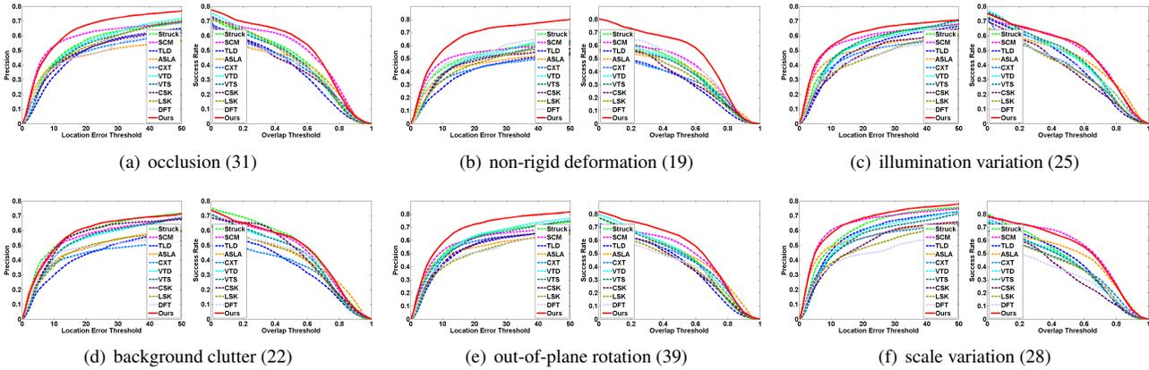
Figure 7. Performance of our tracker and the top ten ranking trackers in [36] in different challenging cases. In the caption of each sub-figure, the number in parentheses denotes the number of the video sequences in the corresponding case.
