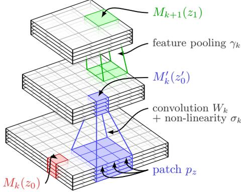
Figure 2. A typical organization for two successive layers of a CNN. The spatial map  $M_{k'}$  is obtained from  $M_k$  by convolution and pointwise non-linearity, and the top layer  $M_{k+1}$  is obtained from  $M'_k$  by a downsampling operation called feature pooling. By convention the map  $M_0$  corresponds to the input image  $x$ .
