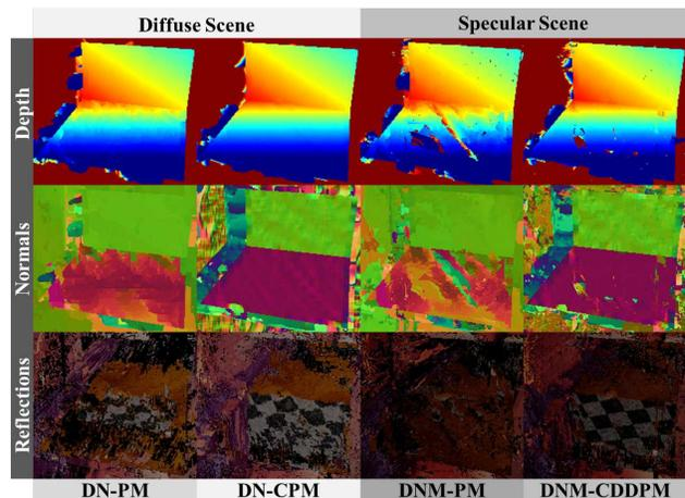
Figure 4. Quality of Normals. **Top to bottom:** depth map, RGB-coded normals and computed reflections. **From left to right:** a) and b) results of DN-PM vs DN-CPM on a diffuse scene. c) and d) result of DNM-PM vs DNM-CDDPM. Inputs are from Fig. 2
