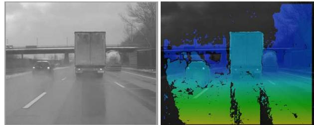
Figure 1. Illustration of Errors Caused by Reflective Surfaces. **Left:** Stereo image. **Right:** Typical Disparity Map. The color observed on the road at the reflection of the silhouette depends on the position of the camera. The algorithm therefore assigns erroneous disparity values at this location.
