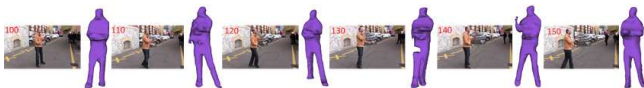
Figure 8. Result for Juggler sequence: Original images from one view with frame numbers and mesh reconstructions alternatively
