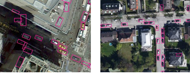
Figure 3. Output of the car detector. This task is challenging due to the small resolution of the target objects. The left image was captured from Google Earth while the right is part of the Bavaria dataset which was used for training the detector.
