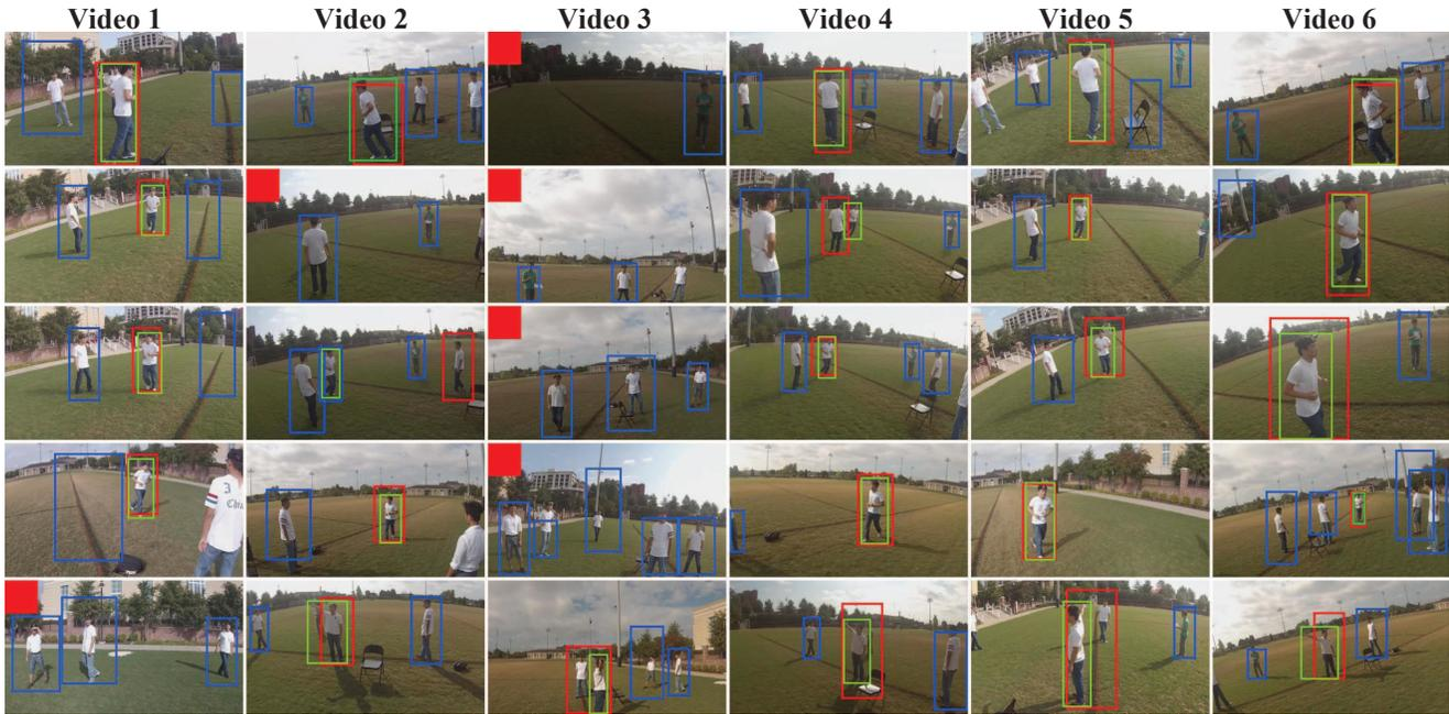
Figure 8. The CIP detection on sample frames from V1. Blue, red and green boxes indicate the detected candidates, the detected CIP and the ground truth, respectively. Frames with a solid red square on the top-left corner indicate that no CIP is detected by our algorithm, e.g., they are drawn from the CIP’s egocentric video or the CIP is occluded in these frames. Frames with a solid blue square on the top-left corner indicate that no candidate is detected in these frames. Best viewed in color.
