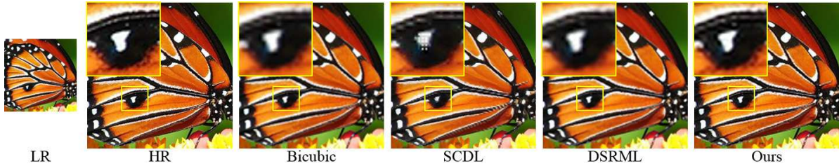
Figure 4. Image super-resolution results of “Red Butterfly” (scaling factor: 2). From left to right: low resolution image, high resolution ground-truth, reconstructed results by Bicubic [12], SCDL [30], DSRML [19] and our approach.
