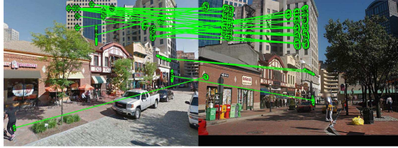
Figure 3: Matching with PBVLAD with similarity threshold 0.5
