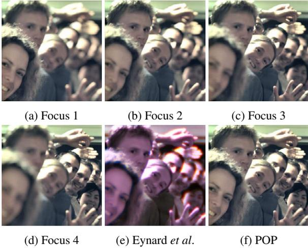
Figure 6: Multifocus Fusion: four color input images with different points of focus captured with one exposure using a plenoptic camera, and the fusion results of Eynard *et al.* and the POP method. The POP result brings details across the image into sharper focus with natural color.
