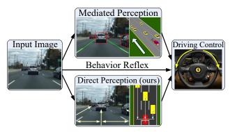
Figure 1: Three paradigms for autonomous driving.
