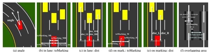
Figure 3: **Illustration of our affordance representation.** A lane changing maneuver needs to traverse the "in lane system" and the "on marking system". (f) shows the designated overlapping area used to enable smooth transitions.
