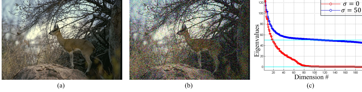
Figure 1. An example to illustrate that patches of a clean image lie in a low-dimension subspace. (a) The clean image. (b) The noisy image with noise \sigma = 50 . (c) The eigenvalues of clean image and noisy image, where the red curve represents the eigenvalues of clean image and the blue curve represents the eigenvalues of noisy image.
