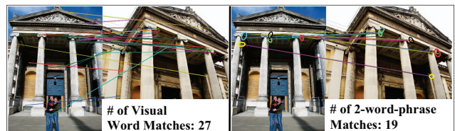
Figure 6. Visual word vs. 2-word-phrases matches between two images of the same object captured from very distinct view points. While word matches require a geometric verification to remove false positive matches, most of the matched 2-word-phrases are true. A few two-word-phrases-matches are highlighted with same-colored ellipses around the keypoint pairs.
