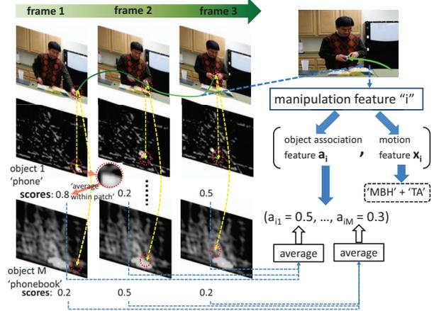
Figure 2. Diagram of computing object association features for a motion trajectory of length  $l = 3$ . Best view in color.
