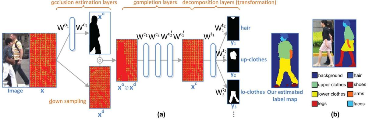
Figure 2. DDN architecture, which combines occlusion estimation, data completion, and data transformation in an unified deep network.
