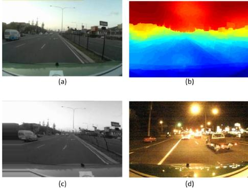
Figure 4: (a) Day-time image, (b) associated depth mask, (c) synthetic sideways shifted viewpoint and (d) corresponding night-time frame from the same location. Note the nearby roadway is not transformed sufficiently due to depth compression issues.
