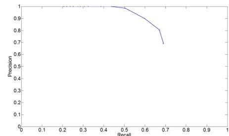
Figure 11: When the synthetic viewpoint system is used, the system achieves a maximum recall of 43.7% at 100% precision, an improvement of 220% over the vanilla SeqSLAM case.
