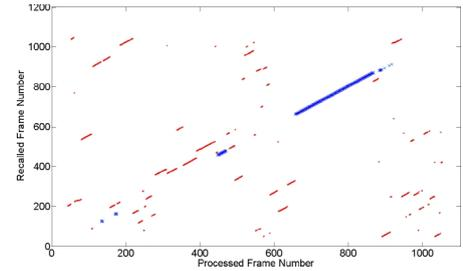
Figure 10: Using vanilla SeqSLAM, the distribution of correct place matches are primarily centered on a region where the day and night traverses were in the same lane, hence removing the requirement for viewpoint invariance (blue cross = true positive place match, red dot = false positive).
