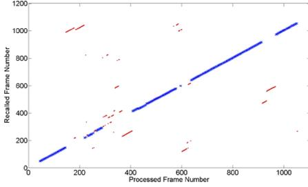
Figure 12: More continuous correct place recognition coverage is achieved over the entire dataset when using synthetic views. The maximum period of incorrect localization is approximately 118 metres.
