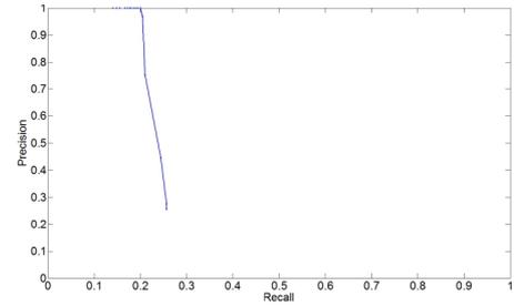
Figure 9: Using vanilla SeqSLAM with image offsetting, a maximum recall of 20% recall at 100% precision is achieved.
