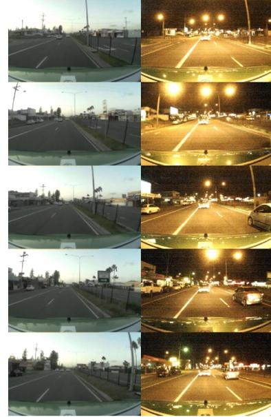
Figure 13: Sample correct place recognition sequence at a one lane offset using the synthetic viewpoint system. This sequence is not correctly matched using vanilla SeqSLAM.
