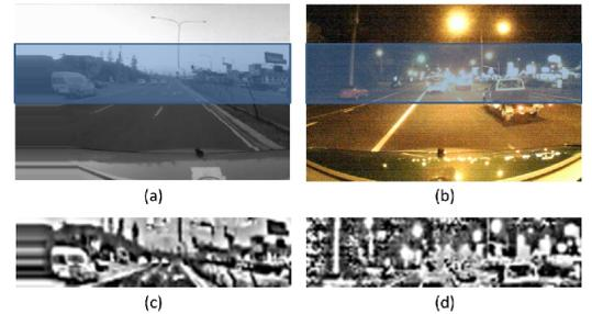
Fig. 8: Original images and low resolution patch-normalized versions used by SeqSLAM
