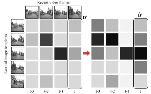
Figure 5: Contrast enhancement of the original image difference vectors increases the number of strongly matching templates. Darker shading = smaller image difference = stronger match.
