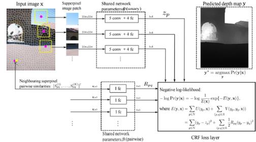
Figure 2: The deep convolutional neural field model for depth estimation (from (Liu, Shen et al. 2014)).
