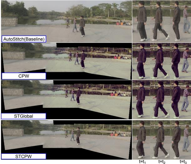
Figure 8. Video stitching results of three RED Scarlet Dragon 4K cameras. **Left:** one of the stitched frames. **Right:** zoomed insets over multiple frames. Note the ghosting and distortion artifacts on the foreground moving objects. Please refer to the supplementary material for stitched videos.
