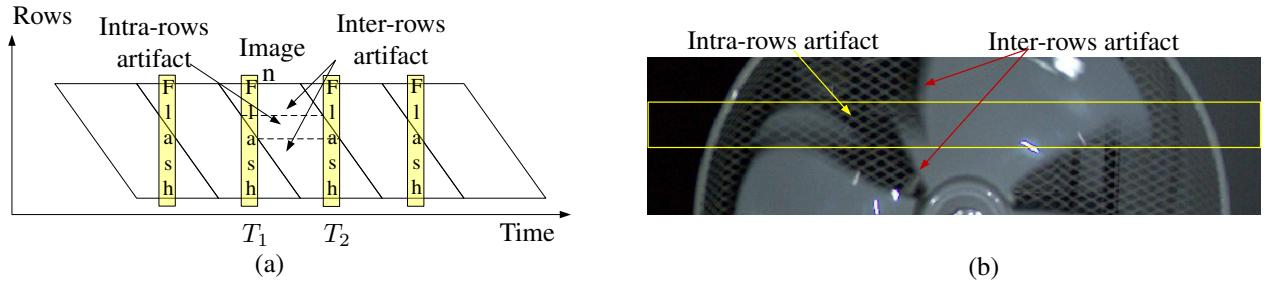
Figure 3: (a): Electronic shutter with periodic flashes, the two types of artifacts are shown in this schema. (b): Typical example of the two artifacts put forward when filming a rolling fan.
