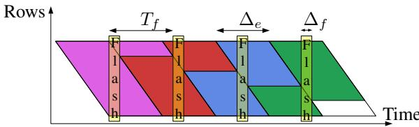
Figure 4: Illustration of the rolling flash method: our method allows to use flashes with electronic rolling shutter camera, fixing the stroboscopic period of flash to the sum of the exposure time  $\Delta_e$  and the flash duration  $\Delta_f$ .
