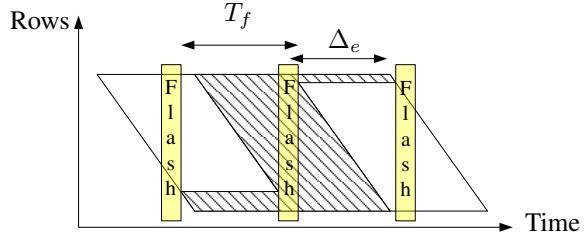
Figure 7: Flash illuminating three frames.
