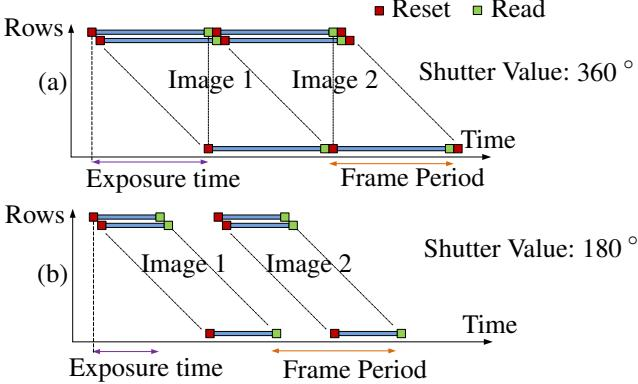
Figure 2: Electronic shutter functioning: a red square represents the reset of a pixel while a green squares represents reading times. (a) For a  $360^\circ$  shutter value and (b) for a  $180^\circ$  shutter value.
