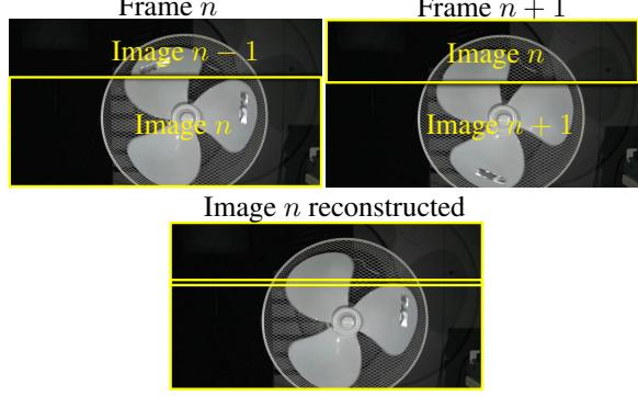
Figure 6: Example of reconstructed image: Image  $n$  is reconstructed from frame  $n$  and frame  $n + 1$ .
