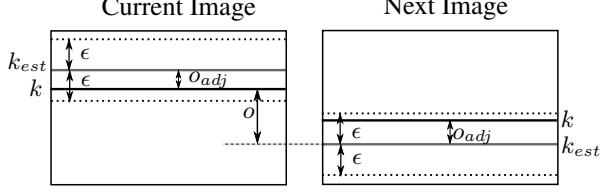
Figure 8: Computing the index  $k$  of the minimal luminance energy row for the current and subsequent images.  $k$  is determined within the range  $[k_{est} - \epsilon, k_{est} + \epsilon]$ . For our experiments we chose  $\epsilon = \frac{h}{100}$ ,  $h$  being the height of a frame.
