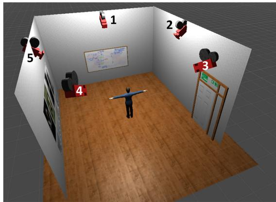
Figure 1. A seminar room simulated in Unity3D<sup>©</sup> with 5 ceiling-mounted cameras in a pentagonal arrangement (cameras are numbered accordingly). A single omni-directional light source was used to illuminate the entire room. For visualization, this light source has higher intensity than shown in Figs. 2 and 3.
