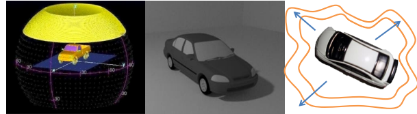
Figure 2. The image synthesis model (left), sample image (center), and acoustic attenuation model (right) for the CVDOME data set.
