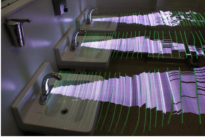
Figure 3. **Visualizing Computer Vision and Seeing How it “Sees”.** Abakography used to indicate spatial extent and view of the sightfield from faucet sensors. Note some degradation of the sightfield farther away from the sensors. Here the test lightfield,  $\beth$ , is indicated by green, and the sightfield,  $\aleph$ , is indicated by the color white.
