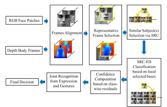
Figure 2. The workflow of our framework. After selecting representative frames from aligned frame sequence, we apply subject selection for a given testing subject. Affection class is recognized for testing queries with selected training data using sparse representation based classification. Then a joint decision from expression model and body gesture model is made based on confidences calculated from class-wise reconstruction residuals.
