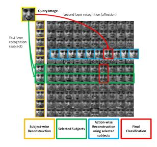
Figure 5. Illustration of our two-layer affection recognition framework. The first layer is to select a subset of subjects which can best approximate the query image(s). The selected rows (colored as green) are used for second-layer affection recognition using SRC. The action-wise approximations are colored as blue. The final decision is to find which class can best approximate the query image. The final decision are shown in red.
