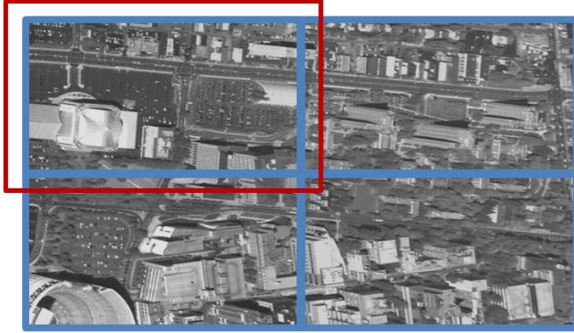
Figure 3. Parallel estimation of tracks and motion patterns on a cluster of computers is enabled by creating an overlapping grid of tiles.
