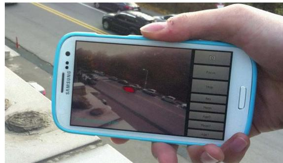
Figure 1. Example of the proposed method running on a mobile device (foreground pixels highlighted in red). Our implementation runs approximately 20 frames per second, comfortably in realtime.
