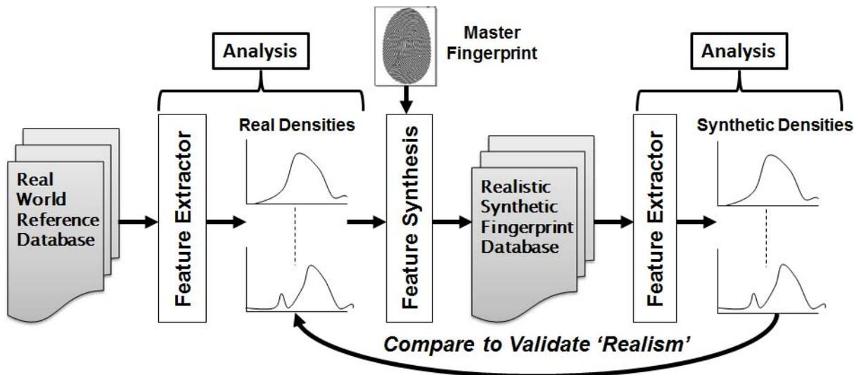
Figure 1: Analysis-by-synthesis process for synthetic fingerprint generation.
