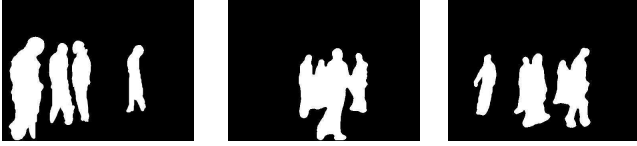
Figure 6. Some “easy” and difficult registration situations. Left: easy scene since blobs are separated. Middle and Right: people are occluding each other, leading to wrong disparity calculations.
