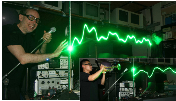
Figure 10. The SWIM's multicomponent/arbitrary waveform lock-in amplifier. Square wave visualized using multicomponent reference signal \cos(\omega t) + \cos(3\omega t) making visible the first two terms of its Fourier series expansion, resulting in phenomenological augmented reality display of \cos(\omega t) + 1/3 \cos(3\omega t) on 600 LEDs in a linear array rapidly swept back and forth on the railcar of an optical table. This suggests expanding the principles of compressed sensing[8, 18] to metaveillance. Inset image: use beyond veillance, e.g. atlas of musical instruments (trumpet pictured) and their waveforms. Amplifiers in picture: SR865 (drifty with screen malfunction); SR510; and PAR124, not used at this time.
