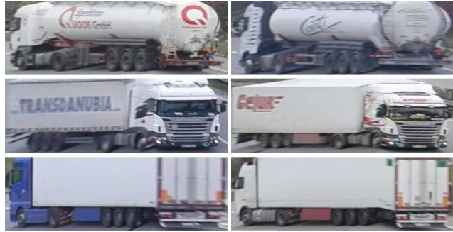
Figure 14. Examples of pairs wrongly identified as identical by the algorithm. The differences are very subtle and difficult to cover by the simple (and fast) linear model.
