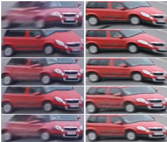
Figure 10. Randomly generated positive pairs of the same vehicle for the linear classifier training. left: Camera A, right: Camera B.
