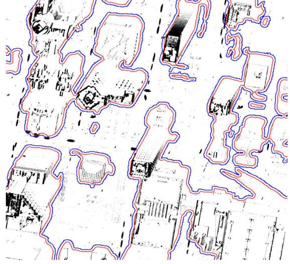
Figure 4. Improved building mask using level-set based geodesic active contours: blue lines are the initial building contours which are evolved and stopped at building actual boundaries (red lines).
