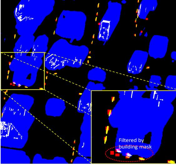
Figure 3. Illustration of motion detection results: true motion detection produced by flux tensor (in yellow color) and false detection caused by parallax in white color. The areas with high altitude are filtered by building mask and are shown in blue. Provided ground-truth bounding-boxes are shown in red.
