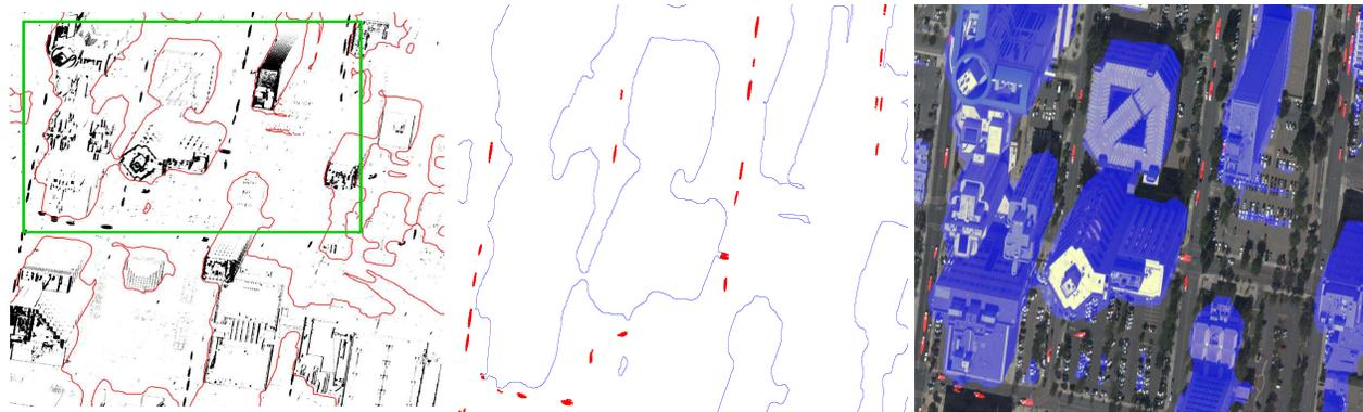
Figure 7. Moving object detection results using the proposed semantic fusion-based approach. The evolved building contours are shown in red in the left most image. The final moving object detection results of the region bounded in green box are shown in middle in red and final building contours in blue. Results are superimposed on the original image where building masks are shown in blue.
