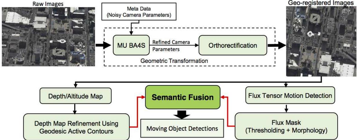
Figure 1. Semantic fusion-based moving vehicle detection system pipeline.
