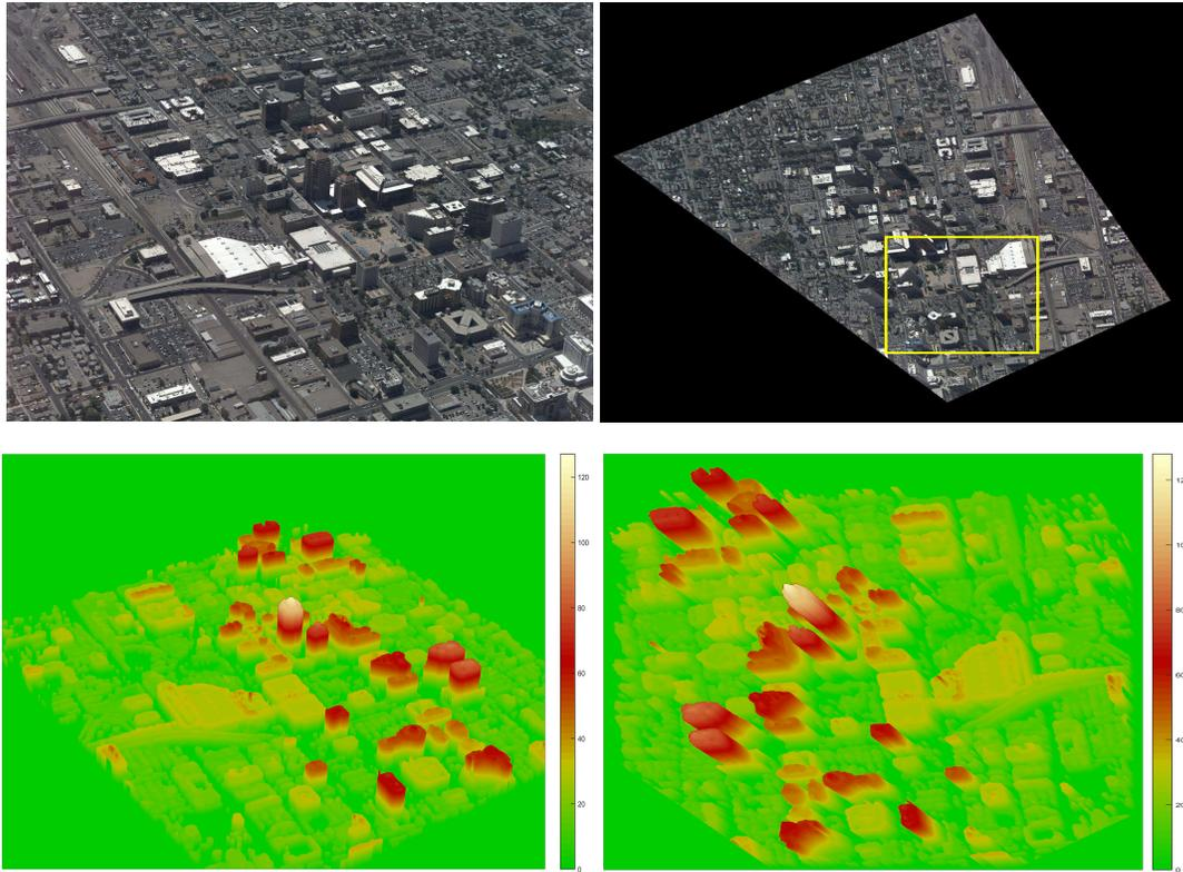
Figure 2. (UL) Illustrates raw ultra high resolution images ( $\sim 30$  MB, each) collected from an airborne platform flying over downtown Albuquerque-NM. (UR) shows the corresponding registered images exploiting *BA4S* orthorectification approach, (LL) corresponding raw image depth mask and (LR) shows the corresponding orthorectified depth mask.
