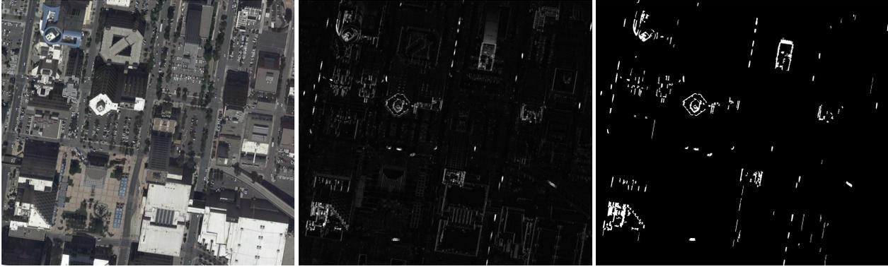
Figure 5. Illustration of motion detection using trace of flux tensor only: From left to right, cropped ROI of Albuquerque aerial imagery ( $f_{r_{100}}$ ), the spatio-temporal motion information computed by trace of flux tensor for the selected image, and flux tensor mask in which each pixel is identified as moving or stationary by thresholding the trace of flux tensor. Morphology is applied to improve the result.
