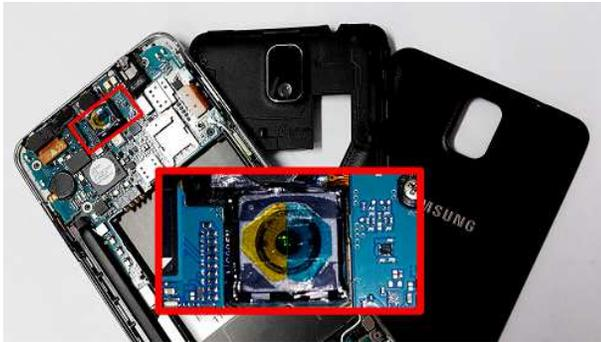
Figure 13. Color-coded aperture smartphone based prototype.
