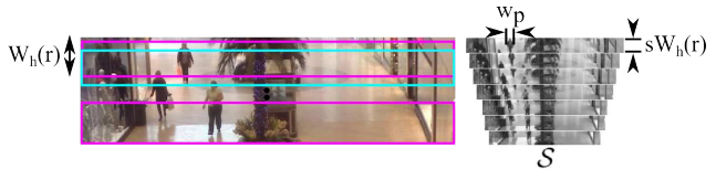
Figure 2: Scale normalization: each video frame is broken into overlapping strips of height W_h(r) (the height of person at a given image row r ) and re-scaled such that the person width in each strip goes to w_p pixels.
