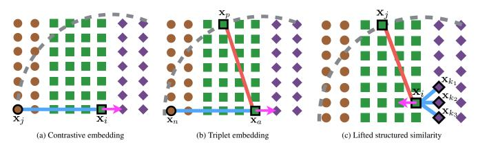
Figure 4: Illustration of failure modes of contrastive and triplet loss with randomly sampled training batch. Brown circles, green squares, and purple diamonds represent three different classes. Dotted gray arcs indicate the margin bound (where the loss becomes zero out of the bound) in the hinge loss. Magenta arrows denote the negative gradient direction for the positives.
