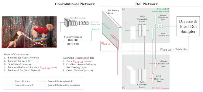
Figure 2: Architecture of the proposed training algorithm. Given an image, and selective search RoIs, the conv network computes a conv feature map. In (a), the *readonly* RoI network runs a forward pass on the feature map and all RoIs (shown in green arrows). Then the Hard RoI module uses these RoI losses to select B examples. In (b), these hard examples are used by the RoI network to compute forward and backward passes (shown in red arrows).
