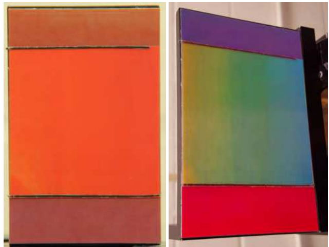
Figure 1. A calibration object made from 3 lenticular arrays. Each lenticular array has an observed color that changes depending on its viewing angle. (Left) When viewed from reasonably far away, the arrays have relatively consistent colors because they are being viewed from approximately the same angle. (Right) A wide angle view from much closer has significant color variation because the direction from the camera to different parts of the object varies substantially. This paper uses this color variation to derive strong geometric constraints for simultaneous, single-image pose estimation and camera calibration.
