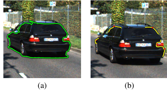
Figure 2. (a) A long level line that forms the boundary of an object. The information present along such level lines is discarded by MSER. (b) A few corners (marked in red) detected by us on locally stable portions of the level lines .
