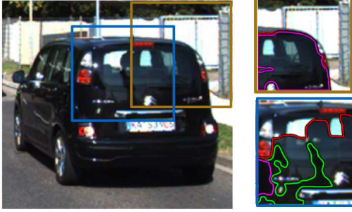
Figure 3. Stable and Unstable level lines in brown (top right) and blue (bottom right) boxes respectively. The Green level line \mathcal{L}\mathcal{L} is tested by considering \mathcal{L}\mathcal{L}_{\mathcal{N}}(\mathcal{L}\mathcal{L}, \delta) and \mathcal{L}\mathcal{L}_{\mathcal{N}}(\mathcal{L}\mathcal{L}, -\delta) level lines in red and purple respectively. Note that the lines are very close in the brown box due to which they mostly overlap in the illustration.
