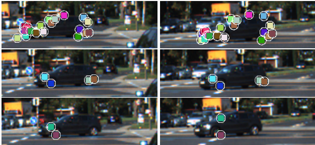
Figure 7. Frame numbers 88 and 93 in the sequence Car-B from the KITTI dataset showing CoMaL + SSD matches in the first row followed by next performing combination: Hessian + SIFT and FAST + NSD in the 2nd and 3rd rows respectively. CoMaL points are matched more numerous and accurately at the object boundary regions in spite of a significant change in the background.
