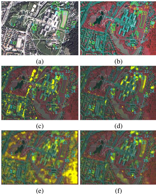
Figure 8. (a) Image in domain  $\mathcal{A}$  and (b)  $\mathcal{B}$ . Change GT marked in green. (c-f) The low confidence areas, those contributing the most to the MRF energy, are shown in yellow. The matching has been performed with the same parameters using the following features: (a) common spectral bands, (b) SIFT, (c) SDSN and (d) SDSN+SIFT. Best viewed in color.
