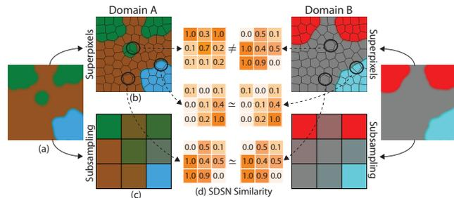
Figure 1. Illustration of Spatial Distribution of Spectral Neighbors (SDSN). (a): Remotely sensed image  $I_A$  in domain A. (b): Superpixels computed for  $I_A$ . (c): Downsampled version of  $I_A$ . (d): The SDSN features are computed as similarities of a superpixel in (b) with every value in (c). The same procedure is applied to the image in domain B. Superpixels belonging to the same land-cover class tend to have similar SDSN values across domains.
