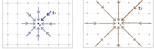
Figure 2: Aggregation from different directions, each direction is decomposed into Markov chains of various spatial step sizes.
