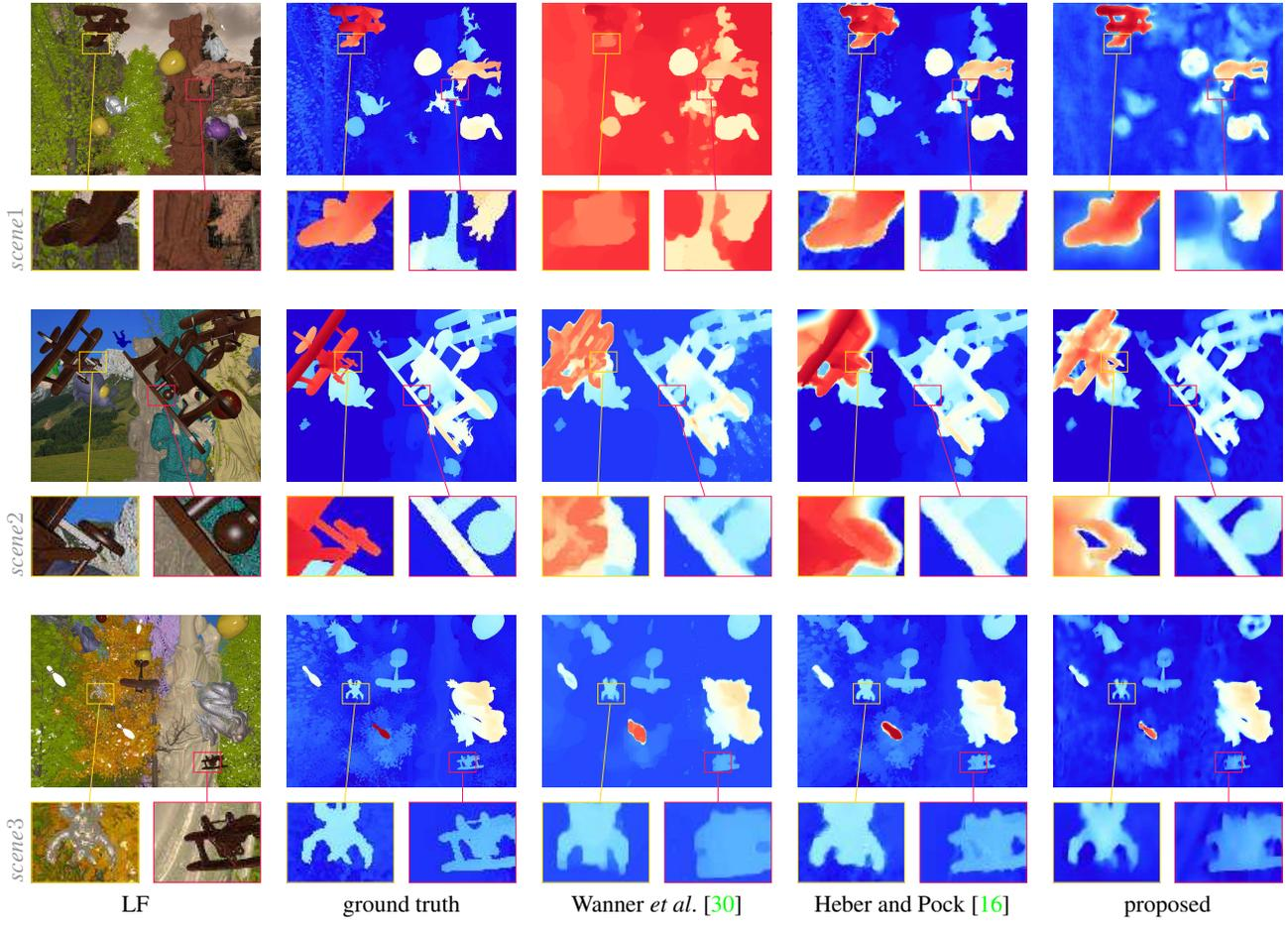
Figure 7. Comparison to state-of-the-art methods on the synthetic POV-Ray dataset. The figure shows, from left to right, the center view of the LF, the color-coded ground truth, the results for two state-of-the-art SflLF methods [30, 16], followed by the refinement result of the proposed method.
