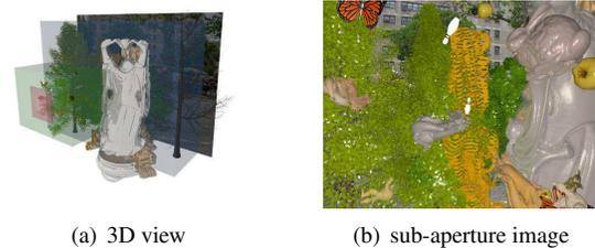
Figure 4. Illustration of a rendered LF. (a) provides a 3D view of a randomly generated scene, where foreground, midground, and image plane are highlighted in green, blue and purple. (b) shows a sub-aperture image of the obtained LF.
