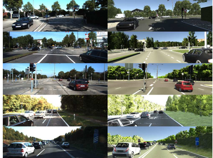
Figure 2: Frames from 5 real KITTI videos (left, sequences 1, 2, 6, 18, 20 from top to bottom) and rendered virtual clones (right).
