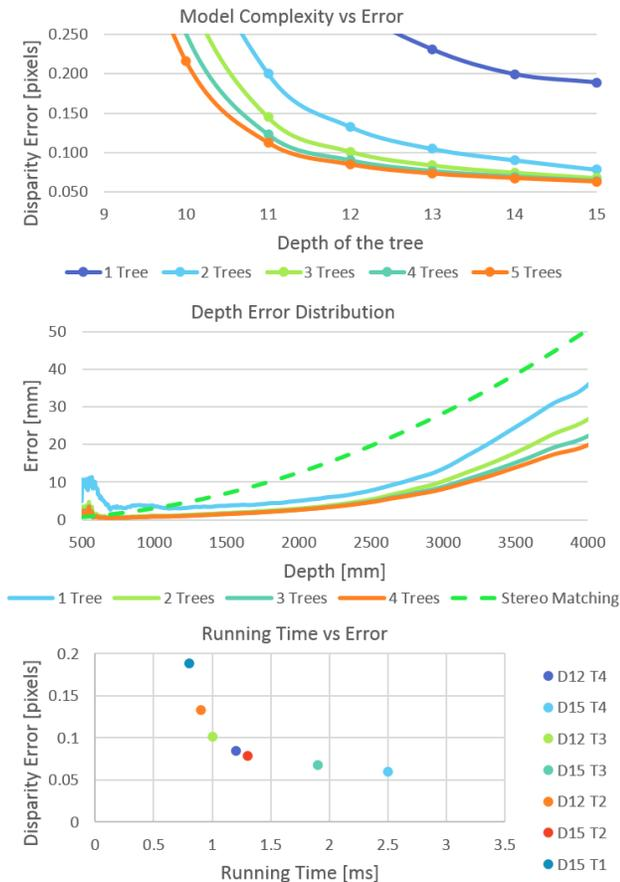
Figure 2. **Quantitative Experiments.** (top) Our disparity error to ground truth (PatchMatch stereo) as a function of number of trees and their depth. (middle) Our depth error to ground truth (PatchMatch stereo) for different numbers of trees. (bottom) Run time of HyperDepth on 1.3 Megapixel images for different tree depths ( $D12$ ,  $D15$ ) and different tree numbers per scanline ( $T1$  to  $T4$ ). The most accurate configuration with 4 trees and depth 15 takes only 2.5msec per image.
