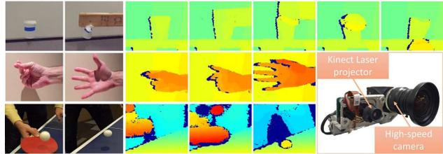
Figure 8. **High Speed Camera Results.** HyperDepth results recorded at 375Hz. (**top**) smashing a paper cup, (**middle**) fast moving hand, (**bottom**) playing ping-pong.
