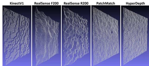
Figure 5. **Plane Fitting Comparison.** We visualize 3D point clouds of a planar target at 1m distance. We compare our results against baseline technologies. Notice the quantization artifacts in KinectV1 and the high noise in the RealSense cameras. Our method and PatchMatch produce smoothest results.
