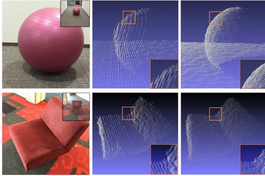
Figure 6. **Quantization Experiment.** We show point clouds generated with KinectV1 (**middle**) and our HyperDepth algorithm (**right**). Notice the heavy quantization in the KinectV1 results, whereas our method infers precise depth.
