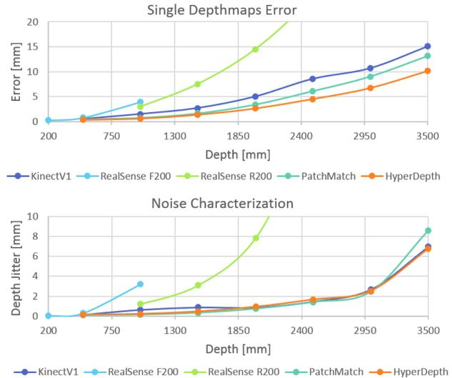
Figure 4. **Error and Noise Analysis.** We plot the depth error of HyperDepth and baseline technologies for a planar target at distances between 20cm and 350cm. The average error of single depth maps is shown on the **top**, whereas the variance within multiple depth maps is shown in the **bottom** figure. Our method exhibits lower error than all baselines.
