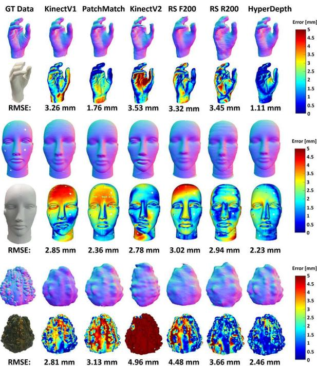
Figure 7. **3D Scanning Results.** Quantitative comparisons between our method and state of the art depth technologies.
