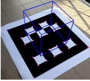
Figure 6: Using ArUco pattern to obtain 2D-3D correspondences. Camera pose estimation allows to place objects in the scene.
