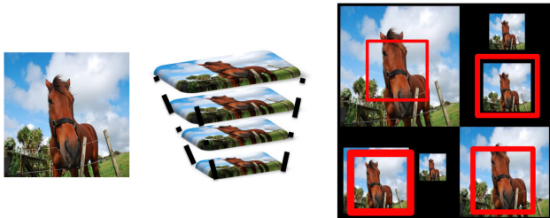
Figure 6. We use image patchworks to efficiently implement scale and position search in DCNN training: an image pyramid is unfolded into an image ‘patchwork’, where sliding a fixed-size window amounts to search over multiple positions and scales. The maximum classifier score on all such windows is efficiently gathered by max-pooling the DCNN’s top-layer responses, accommodating scale and position changes during both training and testing.
