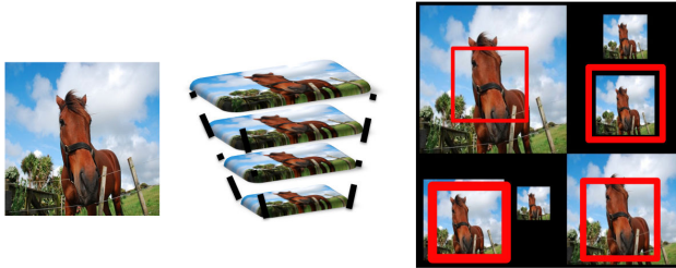
Figure 6. We use image patchworks to efficiently implement scale and position search in DCNN training: an image pyramid is unfolded into an image ‘patchwork’, where sliding a fixed-size window amounts to search over multiple positions and scales. The maximum classifier score on all such windows is efficiently gathered by max-pooling the DCNN’s top-layer responses, accommodating scale and position changes during both training and testing.
