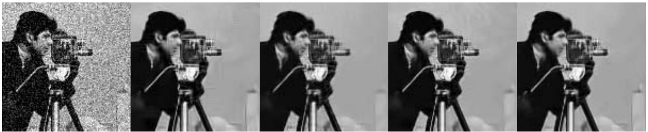
Figure 5. Perceptual comparison for Cameraman . From left to right: (a) Noisy image ( \sigma_n = 30 ); (b) BM3D (PSNR = 28.27dB); (c) LPG-PCA (PSNR = 27.83); (d) CSR (PSNR = 28.54dB); (e) Proposed (PSNR = 28.63dB).
