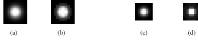
Figure 4. GT blurring kernels and examples of estimated blurring kernels. (a) GT Gaussian blurring kernel with \sigma = 0.6s = 2.4 . (b) An example of estimated blurring kernel of (a). (c) GT Gaussian blurring kernel with \sigma = 0.4s = 1.6 . (d) An example of estimated blurring kernel of (c).
