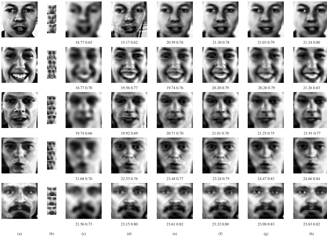
Figure 1. Results of face hallucination using multiple simulated LR faces. (a) HR faces x . (b) LR faces Z obtained by warping HR faces in (a) with random homographies, then blurring with Gaussian blurring kernel with \sigma = 0.6s and sub-sampling by s = 4 to 15 \times 15 , and finally adding Gaussian noise with \eta = 2 . (c) Results of generic HMRF prior in combination with the GT blurring kernel and transformations. (d) Results of PCA prior in combination with the GT blurring kernel and transformations initialized by tracking. (e) Results of PCA prior in combination with an estimated blurring kernel and transformations. (f) Results of PCA prior in combination with the GT blurring kernel and transformations. (g) Results of the proposed patch-wise MPPCA prior in combination with an estimated blurring kernel and transformations. (h) Results of the patch-wise MPPCA prior in combination with the GT blurring kernel and transformations. Number below images is PSNR/SSIM. The images are better viewed by zooming.
