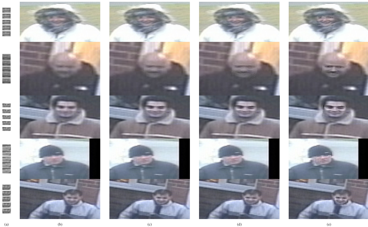
Figure 5. Results of face hallucination in real LR sequences. (a) Multiple LR faces obtained by tracking forwardly and backwardly in sequences. (b) Results of bi-cubic interpolation. (c) Results of generic HMRF prior in combination with a fixed Gaussian blurring kernel with \sigma = 0.4s and transformations initialized by tracking. (d) Results of PCA prior in combination with a fixed Gaussian blurring kernel with \sigma = 0.4s and transformations initialized by tracking. (e) Results of the proposed method using patch-wise MPPCA in combination with an estimated blurring kernel and estimated transformations. The images are better viewed by zooming.
