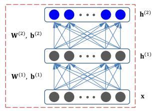
Figure 2. The network architecture used in our method. The input to the network is  $\mathbf{x}$ , and the output of the hidden layer and the top layer is  $\mathbf{h}^{(1)}$  and  $\mathbf{h}^{(2)}$ , respectively. Here  $\mathbf{W}^{(m)}$  and  $\mathbf{b}^{(m)}$  are the parameters of the network to be learned,  $1 \le m \le 2$ .
